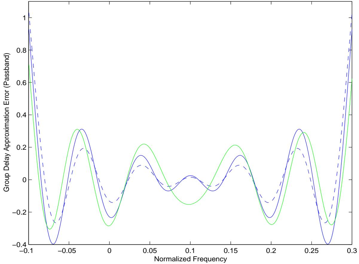
**Figure 4.** Group delay approximation errors inside the passband for the design of a nearly linear phase lowpass complex filter of length 51. Proposed method (solid), Complex Remez (half-tone), don't care region (dashed).
