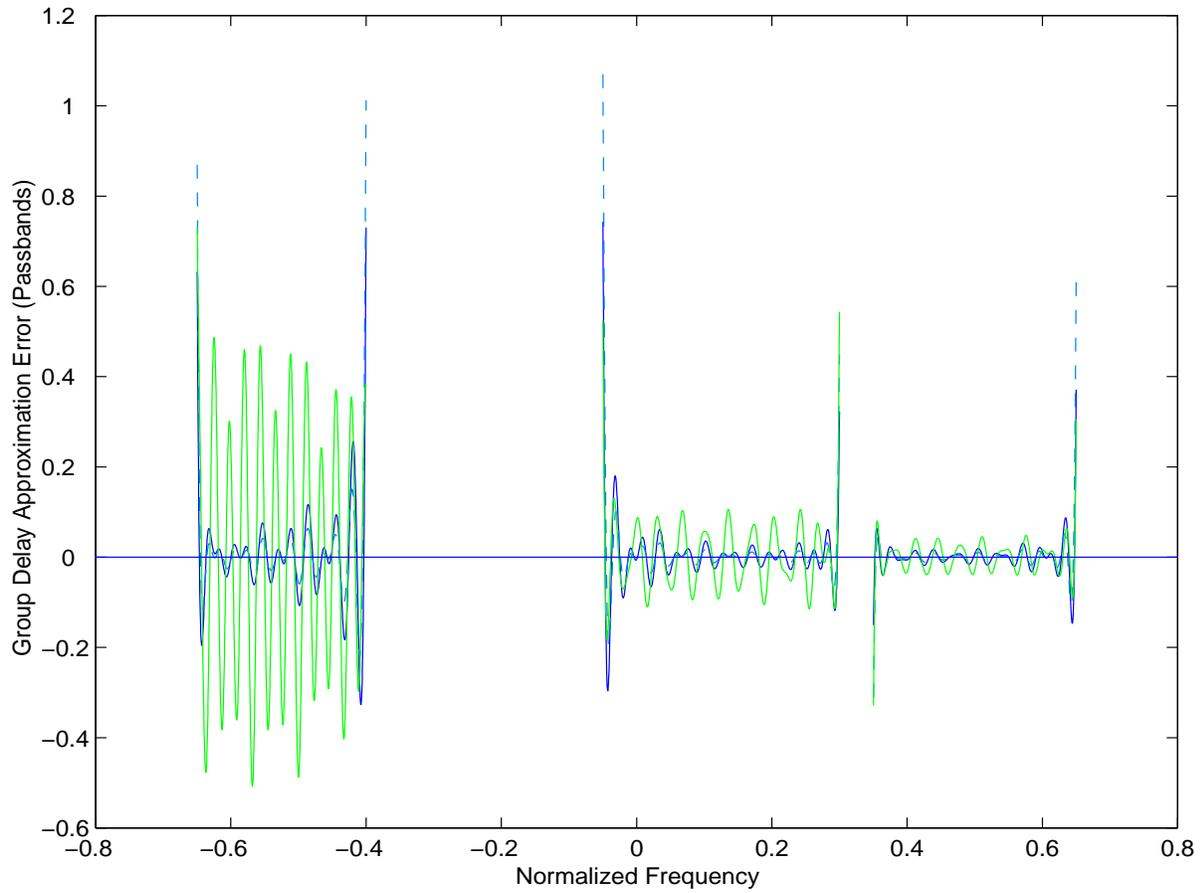
**Figure 8.** Group delay approximation errors inside the passbands for the design of a nearly linear phase multiband complex filter of length 151. Proposed method (solid), Complex Remez (half-tone), don't care region (dashed).
