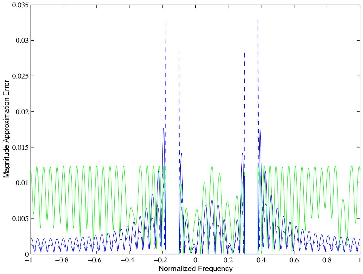
**Figure 3.** Magnitude approximation errors for the design of a nearly linear phase lowpass complex filter of length 51. Proposed method (solid), Complex Remez (half-tone), don't care region (dashed).
