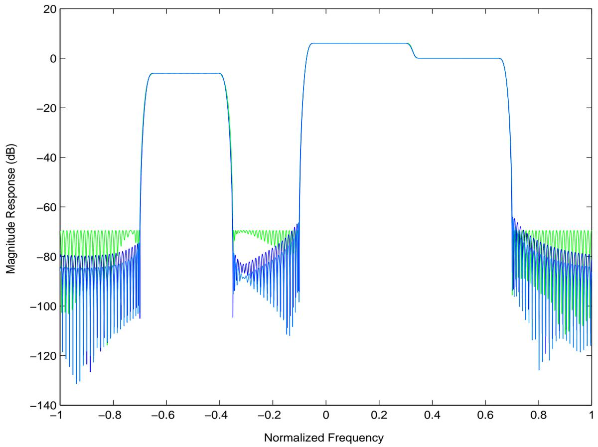
**Figure 7.** Magnitude response of a nearly linear phase multiband complex filter of length 151. Proposed method (solid), Complex Remez (half-tone), don't care region (dashed).
