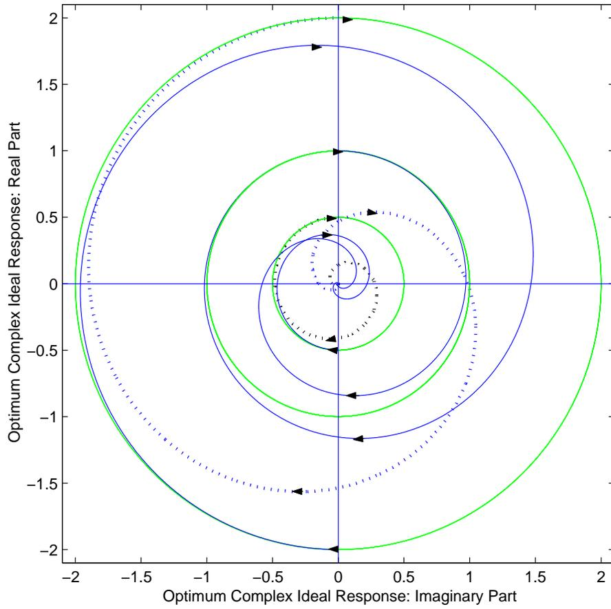
**Figure 6.** Trace of the optimum ideal response of a nearly linear phase multiband complex filter of length 151. Passbands (half-tone), Transitions regions (solid and dotted).
