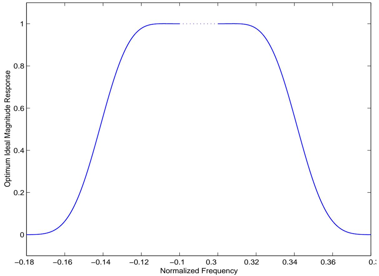
**Figure 1.** Optimum ideal magnitude response for the design of a nearly linear phase lowpass complex filter of length 51.
