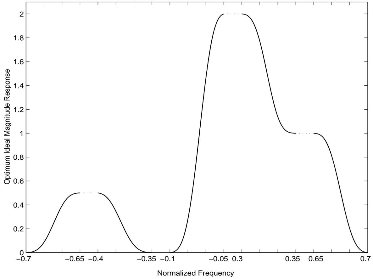
**Figure 5.** Optimum ideal magnitude response for the design of a nearly linear phase multi-band complex filter of length 151.
