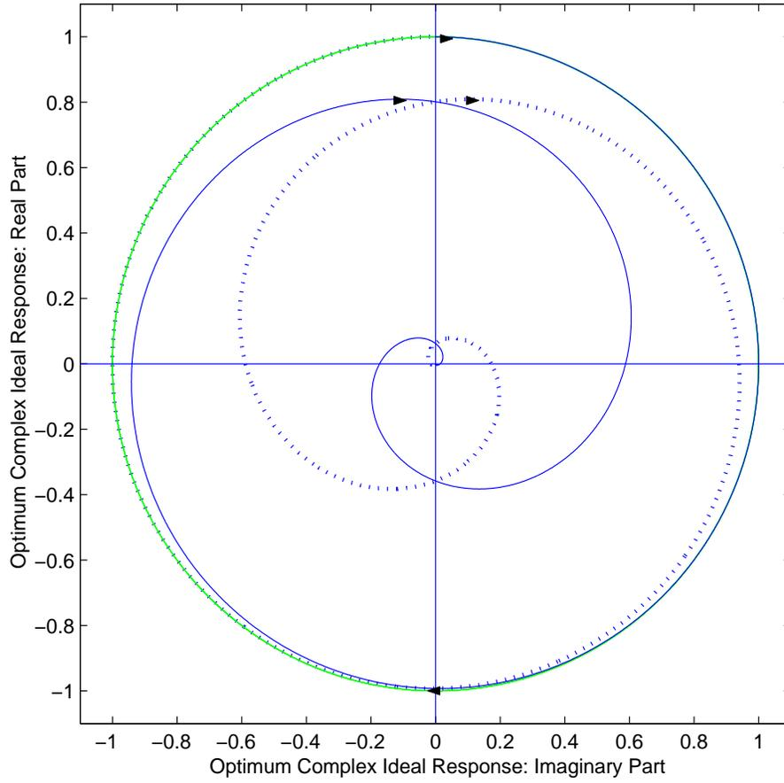
**Figure 2.** Trace of the optimum ideal response of a nearly linear phase lowpass complex filter of length 51. Passband (half-tone), Transitions regions (solid and dotted).
